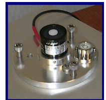
Solar Radiation Sensor
