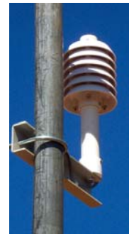
Temperature & Relative Humidity with SUNBLOCK Shield
