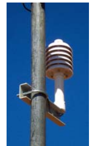
Temperature & Relative Humidity Sensor with SUNBLOCK Shield
