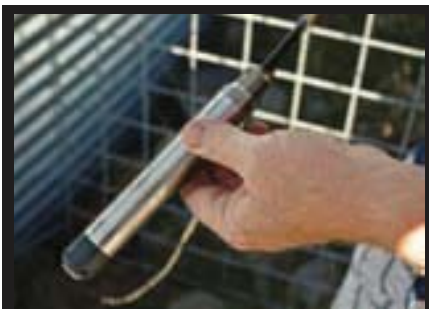
PRESSURE TRANSDUCER: This tool measures water pressure in a tank, which is converted to feet or inches of water left in a collection unit.
