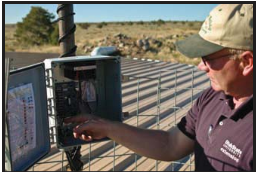
SOLAR AND SATELLITE: This solar-powered livestock water monitor, checked by Utah State University Extension agent Kevin Heaton, sends messages from remote water stocks to the ranch headquarters on water system operations.
